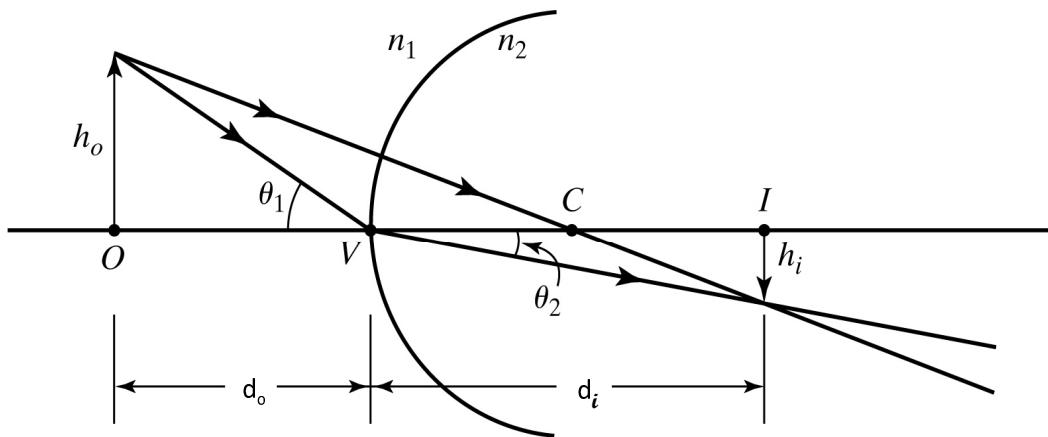
Referring to the figure above, the object is denoted by  $O$ , the image is denoted by  $I$ , the center of curvature of the spherical surface is denoted by  $C$  and the symmetry axis from  $O$  to  $I$  crosses the spherical surface at  $V$ .
